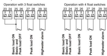
An operation with a joint line of the float switch is not possible.
