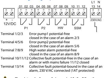
The +/- terminal can only be used with the NA option (mains-independent alarm or 12V battery) up to 1A.
